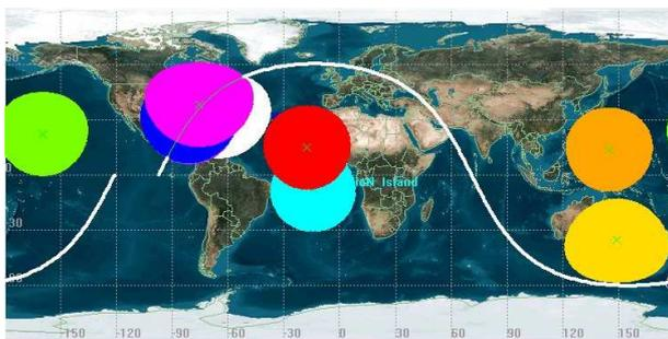
Figure 2: This orbit ground track shows several ground station locations and their ranges. At some locations, the satellite sees several ground stations, whereas, at other locations, the satellite is just barely out of range. Robust capacity-constrained scheduling is aimed at optimizing the transfer of data from space to ground.
