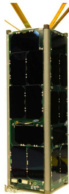
Figure 1: The Radio Aurora Explorer (RAX) triple Cubesat developed for NSF at the University of Michigan.
