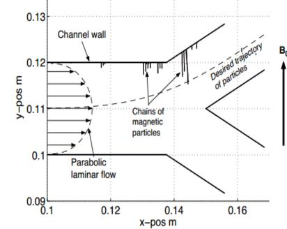
Capillary systems are designed in order to study the ability of guiding magnetic particles through a porous membrane in the presence of a flow. Observations from both experiments and simulations show that aggregates of magnetic particles are moving faster compared to single particles.
