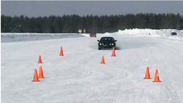
*Platform 1.* The Jaguar in Figure 5 is equipped with active steering, braking and throttling. GPS, accelerometers, gyros and 3D stereo vision. The controllers are run on a dSPACEAutobox system.
