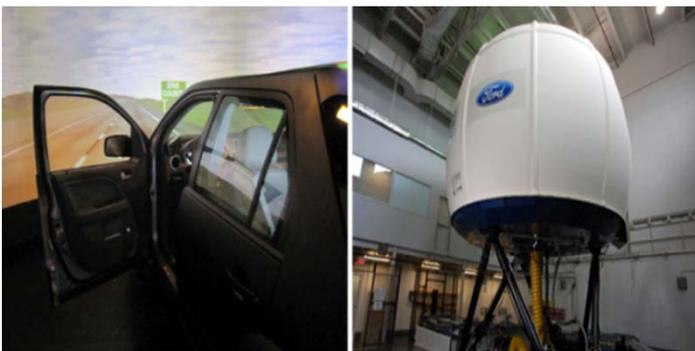
*Platform 2.* The VIRTual Test Track Experiment (VIRTTEX) simulator, pictured on the left, is a spherical dome (with a actual car inside) on top of a hydraulic system to mimic vehicle movement. In addition, it has image rendering technologies to provide a high-resolution, digitally projected 360-degree horizontal field-of-view to test and measure driver acceleration, braking and steering performance as well as overall driver reactions in varying conditions.
