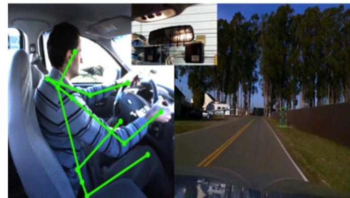
*Platform 3.* The *vehicular test bed* is a car equipped with outward looking and inward looking cameras observing the interior and exterior of the vehicle, illustrated on the left. Drivers will employ the test bed during daylong experiments (in real driving) while the driver's input, the vehicle's state, observations of the driver, and observations of the environment will be recorded for post-
