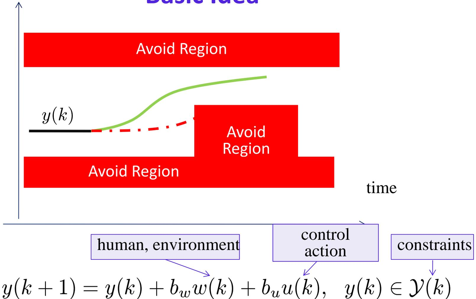
At step  $t$  decide on  $\mathbf{u}(t)$  based on prediction on  $\mathbf{w}(t), \dots, \mathbf{w}(t+N), \mathcal{Y}(t), \dots, \mathcal{Y}(t+N)$
