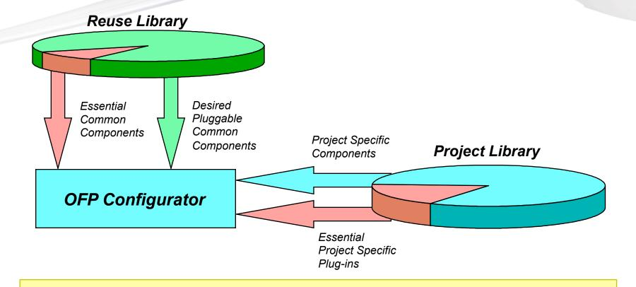
Flight Programs Created Via Component Selection and Wiring
