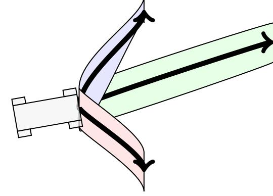
Guaranteed safe and stable maneuver regulation is key to building reliable and robust autonomous vehicles. Our approach treats the control-planning prob lem as a hierarchical structure in which trajectory optimization and maneuver regulation are interwoven, with the possibility for interruption through failure events which would then adjust the controller in response.
