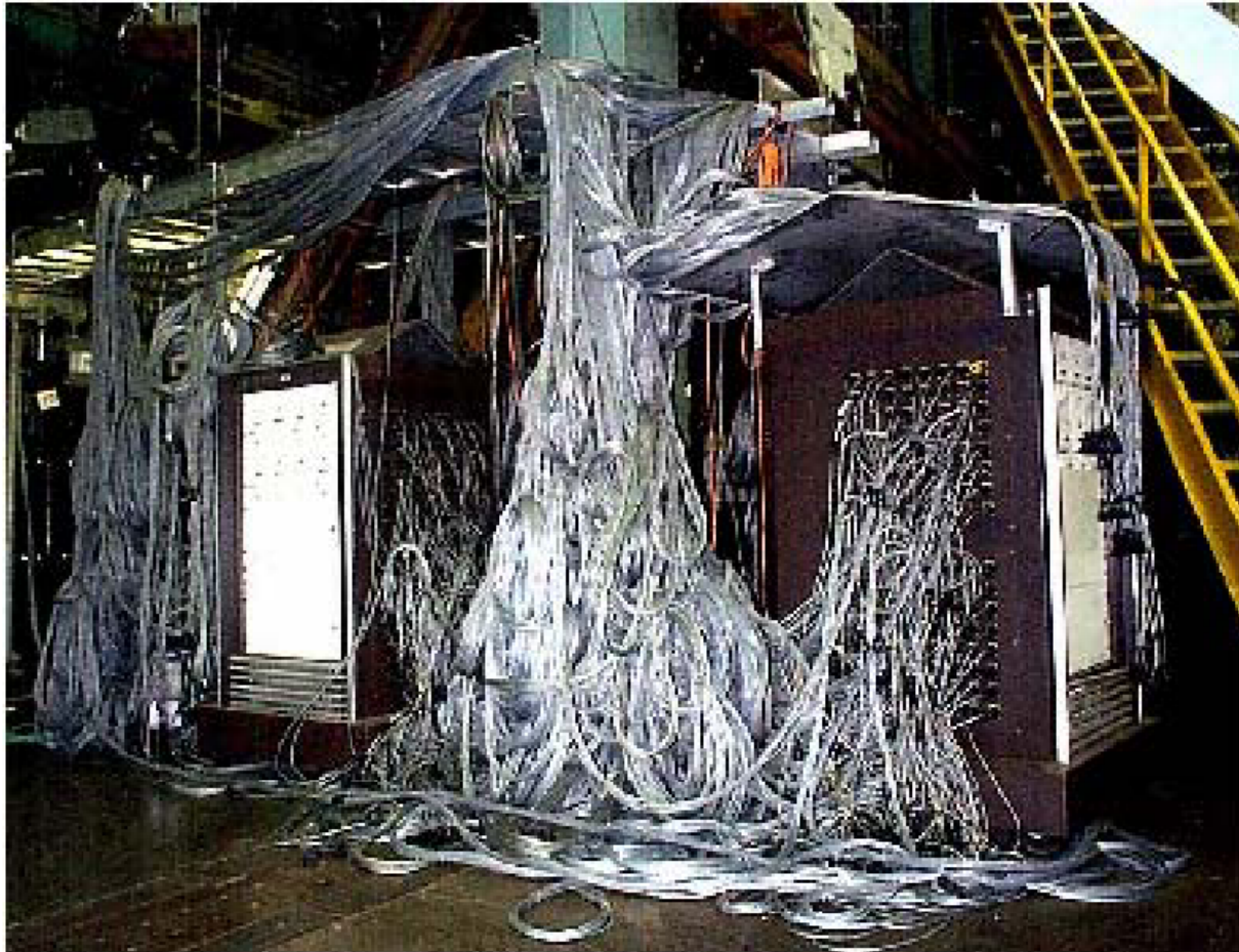
F-18 Aircraft Static Fatigue Test System Boeing
