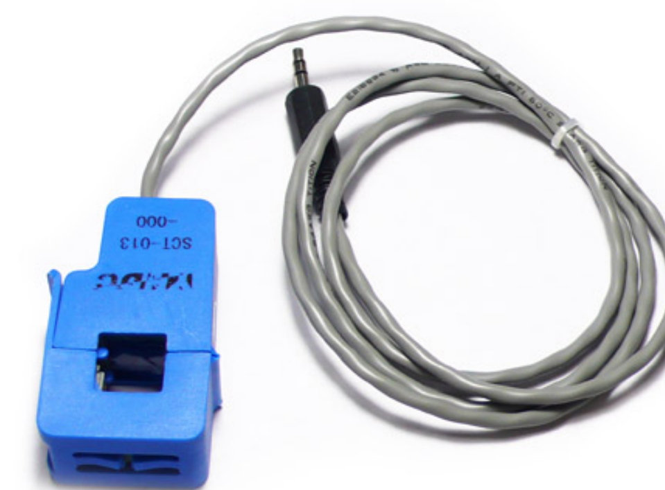
Circuit level monitor
