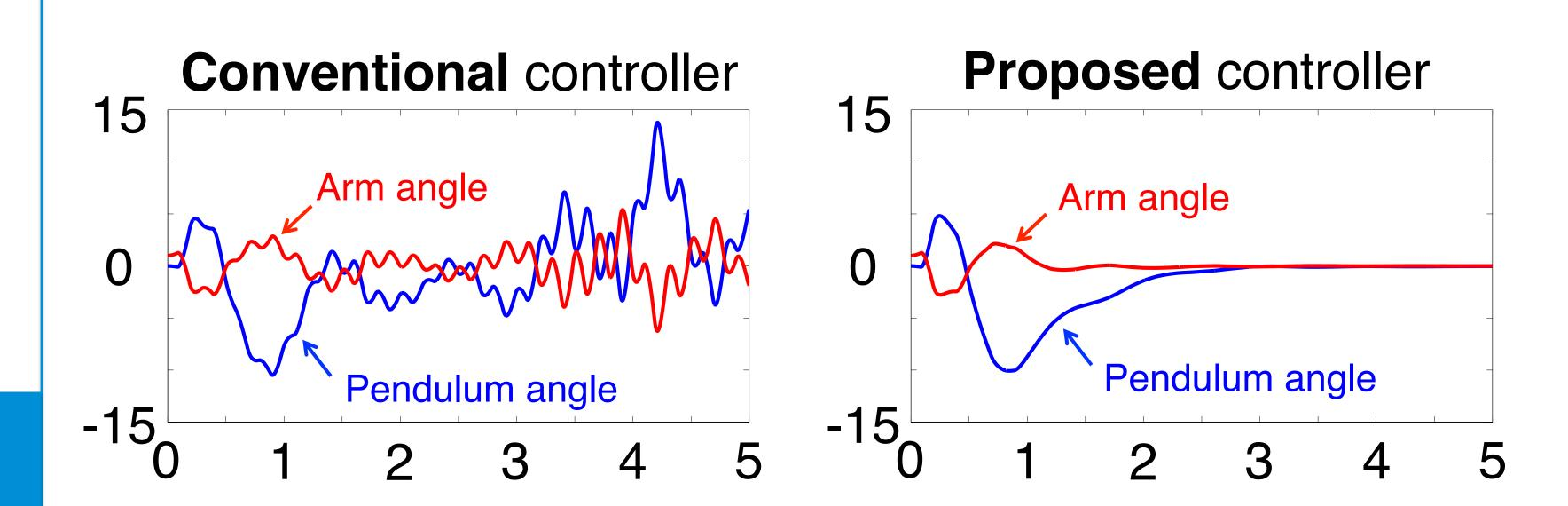
Proposed controller is robust against clock offsets
