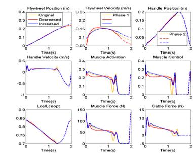
These results show the predicted trajectories obtained by varying the flywheel inertia. The optimal muscle control Strategy is to maintain mostly constant activation during the pull phase, with a sudden jerk at the end to initiate the return motion via the elastic shock cord. In a real human, this would probably not occur because there is an antagonistic muscle, the triceps, which can do this more efficiently.
