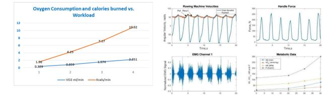
Our team has selected the rowing exercise as a testbed to drive and validate our results. A comprehensive series of tests was conducted in Summer 2016, where machine velocities and forces, as well as extensive physiological data (16-point EMG, oxygen, heart rate and motion marker data at 28 locations) were recorded in nine different experimental conditions.
