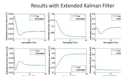
The filters do an almost perfect job of estimating the tendon lengths and CE, assuming that the total muscle length is available for measurement. Note that the filter does an almost perfect job of also estimating the muscle activation levels  $a_i$  (shown in the right plots) even though those quantities are not directly measured.
