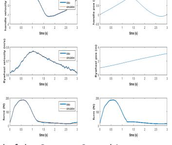
A dynamic model was formulated, and the system parameters were found by fitting the simulation to the experimental data. This was done by direct collocation with periodic boundary conditions for the trajectories.
