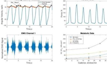
Our team has selected the rowing exercise as a testbed to drive and validate our results. A comprehensive series of tests was conducted in Summer 2016, where machine velocities and forces, as well as extensive physiological data (16-point EMG, oxygen, heart rate and motion marker data at 28 locations) were recorded in nine different experimental conditions.
