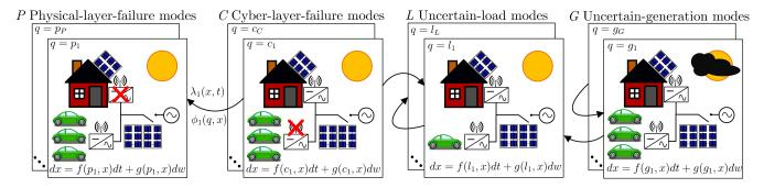
Figure 1: State-transition diagram with illustrative modes and corresponding transitions for CPS failures and uncertain generation/load. Details are hidden in the interest of clarity; e.g.,  $\{g_1, \ldots, g_G\}$  might correspond to G different irradiation levels ( $g_1$  depicts one such irradiation level).
