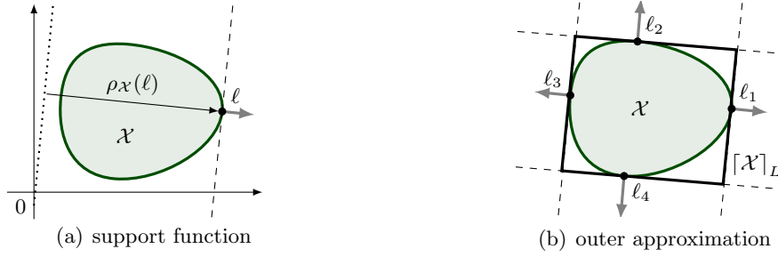
Figure 2: Evaluating the support function in a set of directions gives a polyhedral outer approximation
