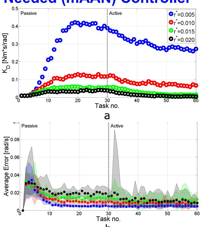
Effect of error bound modification algorithm on feedback gain and average error. (a) Feedback gains for passive subjects (1-30) are higher than for involved subjects (31-60). As the allowable error decreases, the magnitude of robotic assistance increases. (b) The plotted points represent the mean error across all subjects and the shaded regions depict the corresponding variance. As the bound radius increases, subjects display more independence from the given trajectory.
