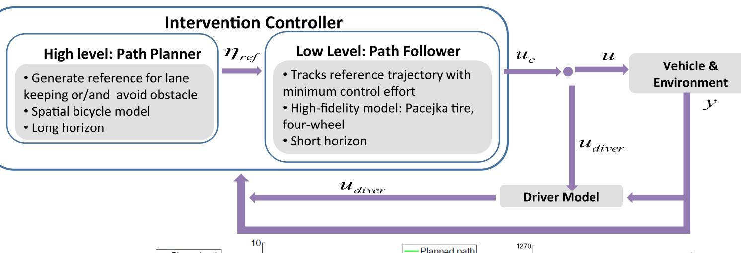
□ Simulation of intervention controller with an existing "simple" driver model, in a road departure scenario.
