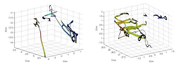
This figure shows the surfaces swept out by a surgical needle operated with a robotic instrument as a subject performs a dry-lab (left) and simulation-based (right) robotic surgery training task.
