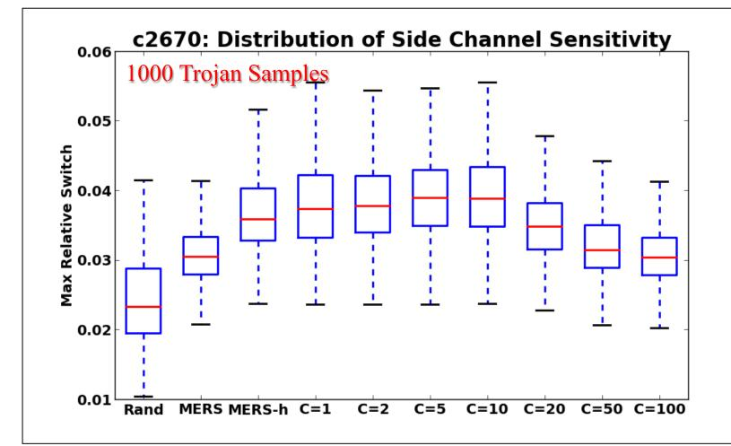
The optimized test patterns MERS-h and MERS-s (with weight C=1 $\sim$ 10) can further increase the side channel sensitivity.
