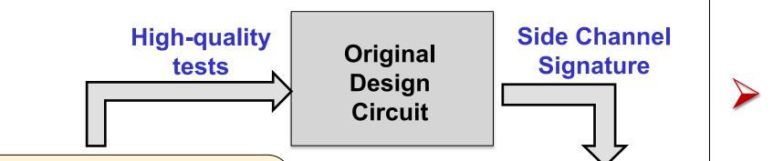
Our statistical approach can improve the sensitivity of side-channel based Trojan detection, by generating high-quality tests.
