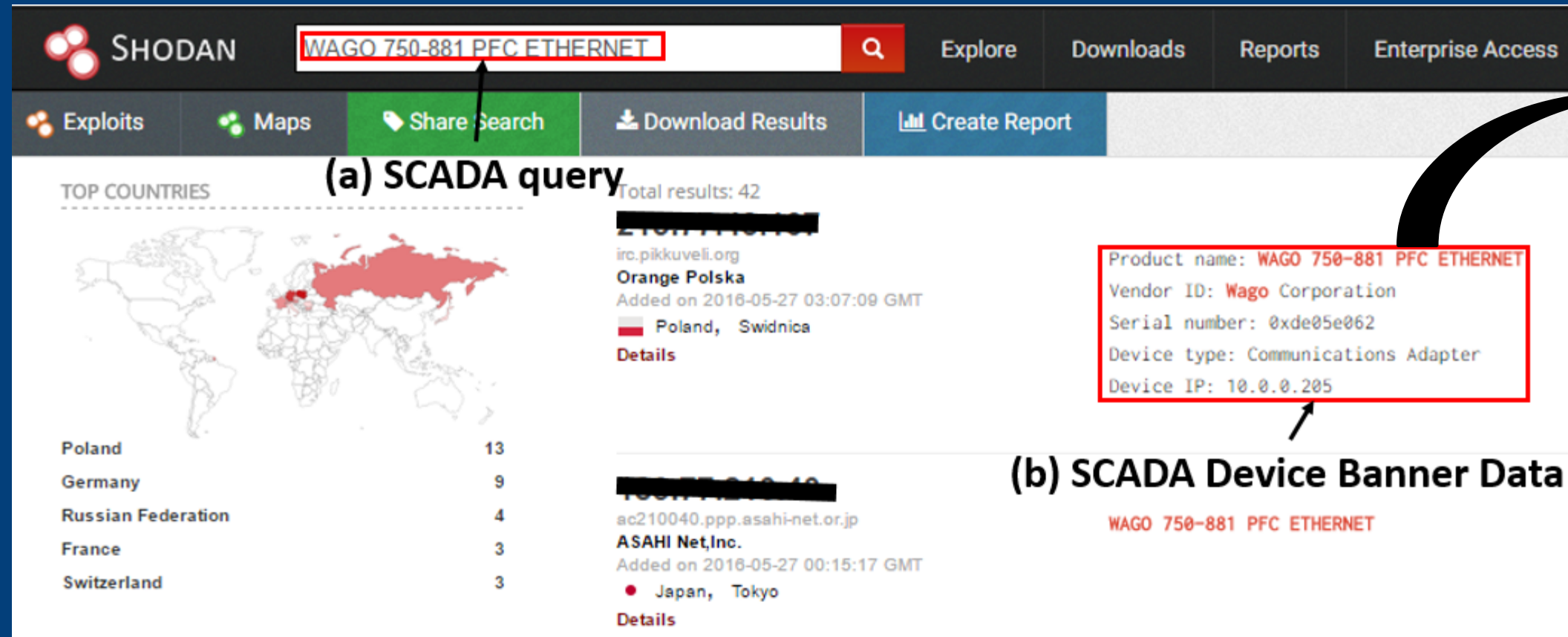
Figure 1. Shodan Results for a SCADA specific Query (WAGO 750-881 PFC)
