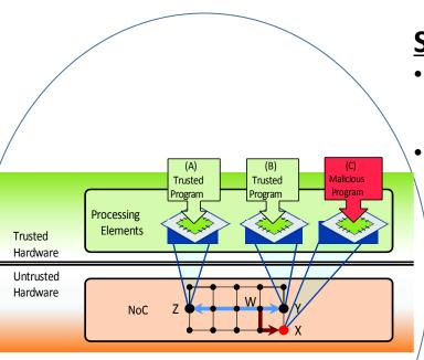
C-NoC snooping data between A & B and leaking to accomplice program C.
