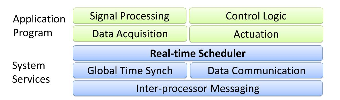
**Control Program Structure**: Control programs are specified as scheduled tasks on multiple controllers.
