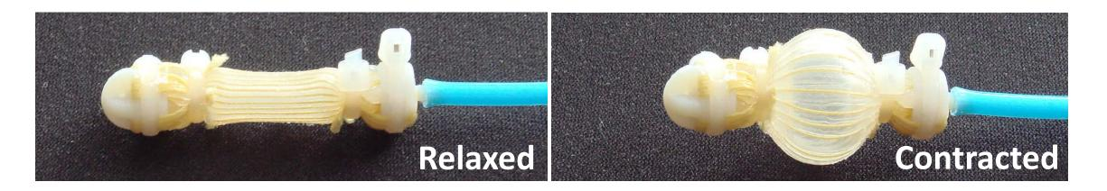
**Sensor**: Each muscle cell is equipped with two strain sensors to measure the contraction of the muscle cell, embedded in the top and bottom layers each. Each strain sensor has an embedded micro-channel filled with liquid metal (EGaIn) that changes overall resistance of the channel as the sensing layer experiences strain changes.
