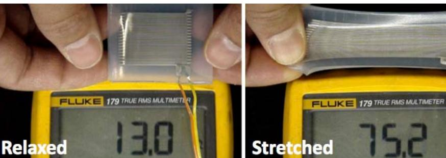
Channel dimension: 200 x 200 μm Nominal resistance: Approx. 10  $\Omega$
