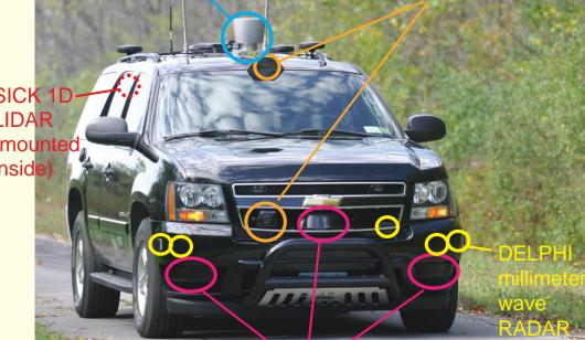
Ibeo LIDAR scanners (4 lasers
