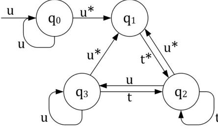
Security automaton design for traffic dependency enforcement in Schneider's EM model [WSCS'12]
