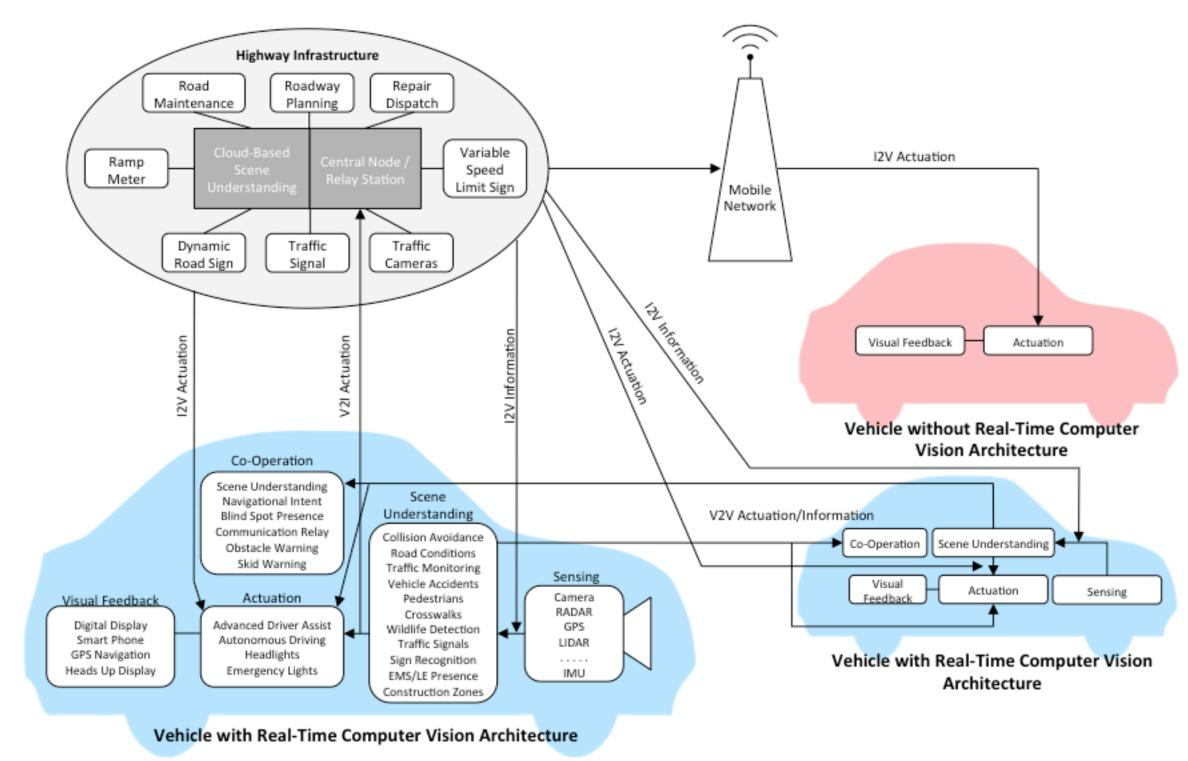
The proposed roadway CPS consists of heterogeneous sub-systems, namely, a vehicle CPS (shown in blue), vehicle-to-vehicle CPS, and a vehicle-toinfrastructure CPS. The sub-systems are capable of sharing rich scene information with each other to ultimately provide useful forms of actuation.
