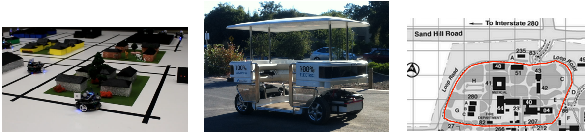
Figure 1: Left Figure: a mock urban environment where 15 small mobile robots provide on-demand service. This test bed allows the validation of dynamic vehicle routing algorithms for automated MOD systems. Center Figure: the NAVIA vehicle to be deployed at the Stanford SLAC Laboratory. Right Figure: the street at SLAC where two NAVIA vehicles will operate (the length of the loop is about 1.5 miles).
