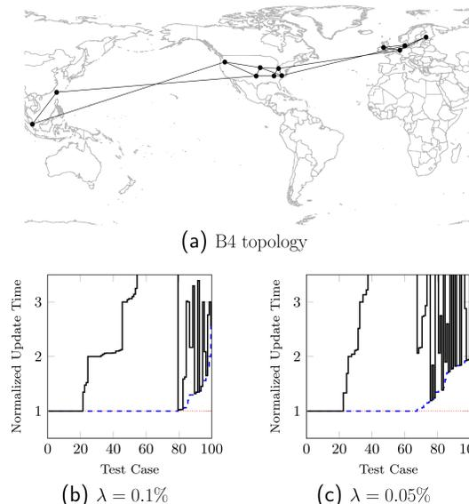
Figure 5: Comparison with SWAN [1], where  $\lambda$  is the scratch capacity rate. Our method not only outperforms SWAN but also achieves near-optimal performance. (blue dashed: our method; black solid: SWAN; red dotted: optimal)
