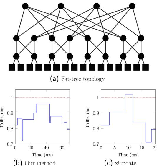
Figure 6: Comparison with zUpdate [2]. Our method ensures the update is congestion-free, while zUpdate may exceed the link capacity under the presence of uncertainty. (the utilization is normalized by the link capacity)
