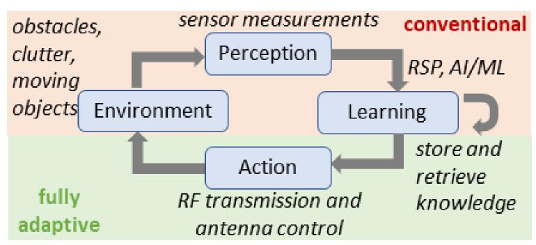
Fully-adaptive RF sensing: RF transceiver can be controlled in a standalone fashion or guided by sensors of other modalities.
