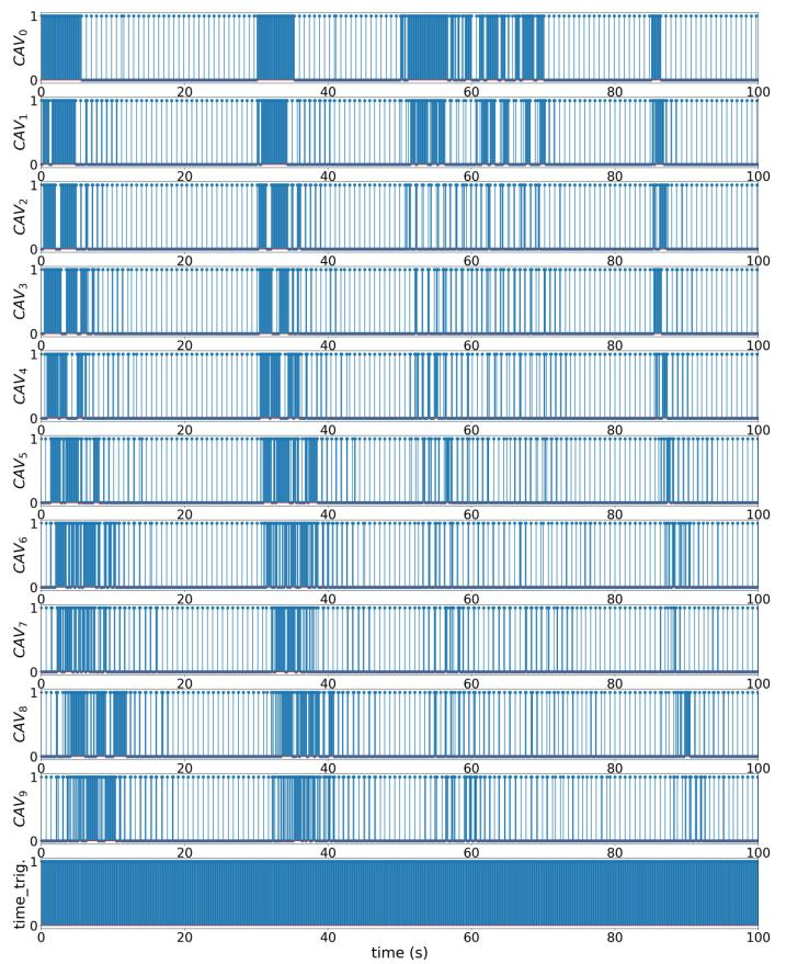
Triggering status of CAVs for eventtriggered MPC (subplots 1-10) and time triggered MPC (subplot 11); eventtriggered noticeably reduces the communication instances for all CAVs.
