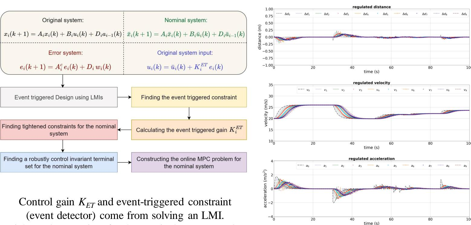
Tightened constraints for the nominal system can be found by knowing gain. Next is to find a robustly control invariant terminal set. Finally, the online MPC problem can be constructed to calculate  $u_i(k)$ .
