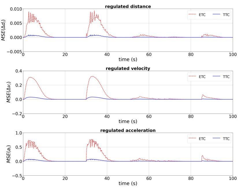
Comparing the mean squared error for two control approaches: event-triggered MPC and time-triggered MPC. As expected, the event-triggered MPC has higher MSE values due to sacrificing performance to achieve less frequent use of communication and computation resources.
