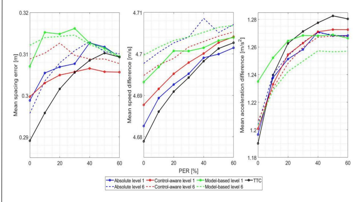
ACC performance (errors) for different communication policies under different loss rates (PER). TTC (fixed comm rate of 10 Hz), absolute triggering ETC (average rate of 4.75 Hz), controlaware triggering ETC (average rate of 5.28 Hz), and model-based triggering ETC (average rate of 1.80 Hz). Level 1 and 6 correspond to tracking error thresholds of 0.1m and 1.1m.
