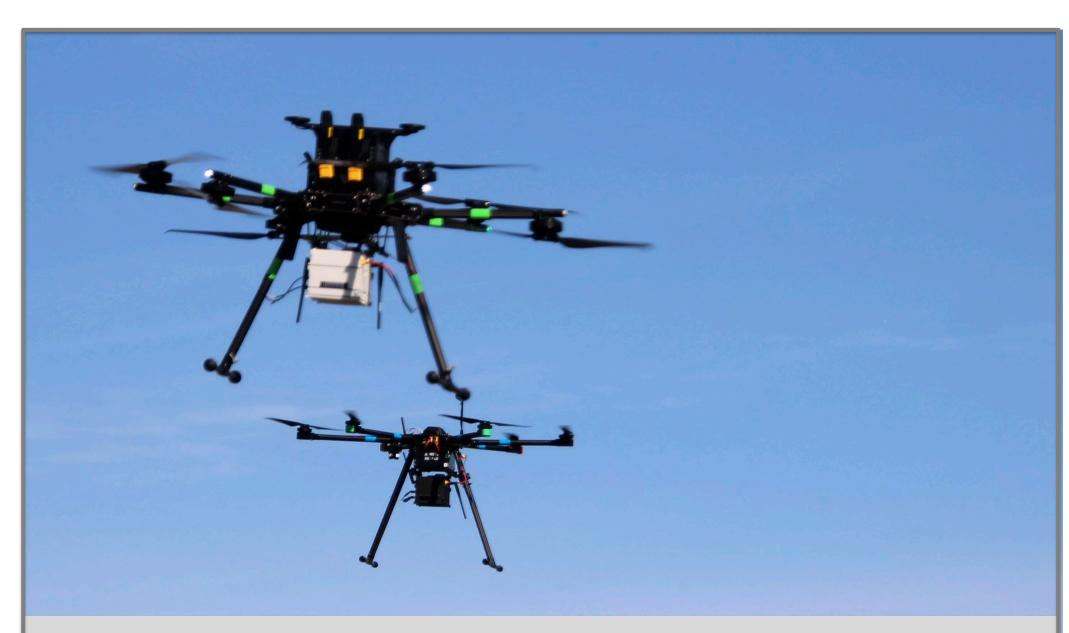
Our air Leasing technology allows drones to operate in shared airspace while maintaining trajectory-aware safe separation distance.
