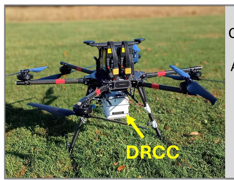
Plug-and-play Control Cubes attach to diverse Px4 and Ardupilot platforms, providing edgebased computing, sensors, power modulation, and mesh radio connectivity.
