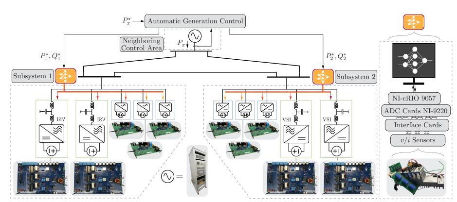
Diagram of hardware testbed with programmable inverters hardware that will act as grid assets. The testbed will contain two subsystems controlled by the proposed learning-based methods embedded within NI modules. A neighboring control area is mimicked with a programmable grid simulator.
