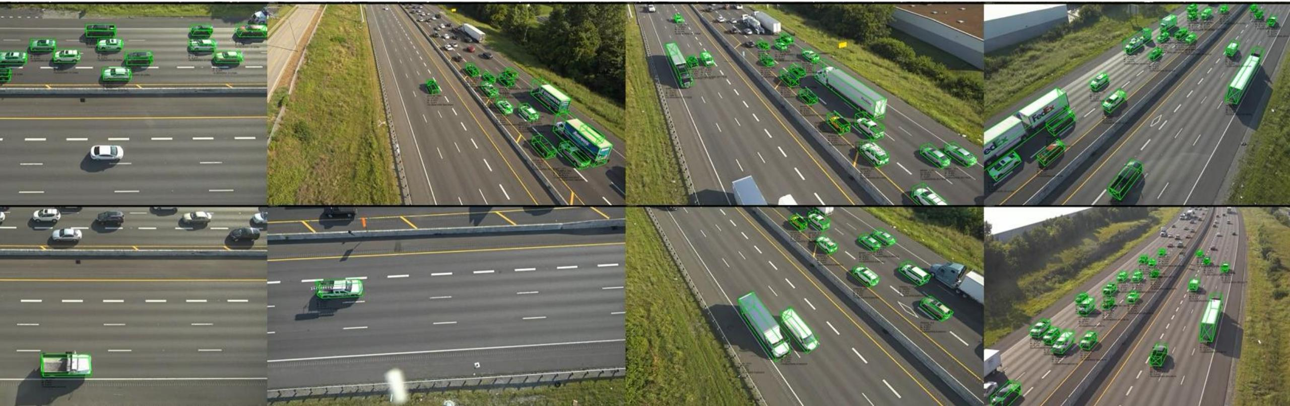
Image space positions are converted to roadway coordinates and stitched across cameras.
