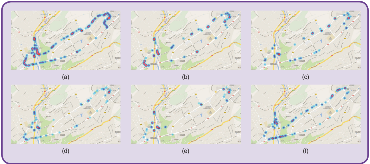
FIG 5 Event locations for the different drivers. (a) Event locations for the aggressive laps. (b) Acceleration event locations. (c) Braking event locations. (d) Event locations for the calm laps. (e) Steering event locations. (f) Overspeed event locations.
