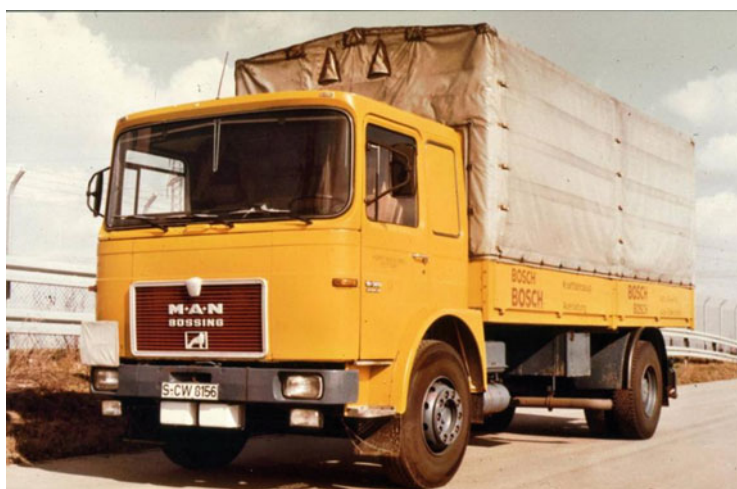
Fig. 10.6 MAN truck equipped with a 35 GHz sensor. Source: private collection of the author
