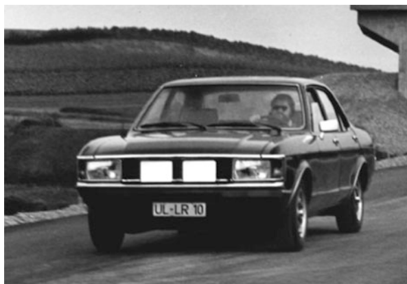
Fig. 10.5 35 GHz automotive radar system built by AEG-Telefunken 1974 (the driver being the 1st author of this paper). Source: private collection of the author
