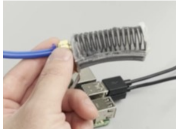
Fiber-reinforced soft finger design
