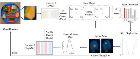
Post hoc augmented contextual bandit framework. We only observe the visual context from SPANet prior to action selection, but the post hoc context from HapticNet is used with the observed loss to update the visual model.
