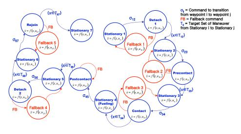
Fig. 3: Aerial Refueling Formation Transition Model. The initial state is Stationary 1.
