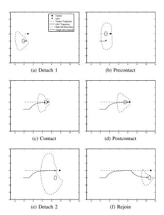
Fig. 5: Refueling sequence simulation with capture sets.
