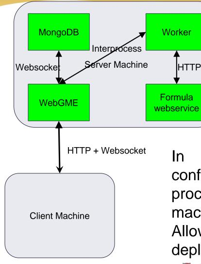
In the smallest deployment configuration all the necessary processes can live on the same machine on the server side. Allowing a quick yet fully functional deployment.
