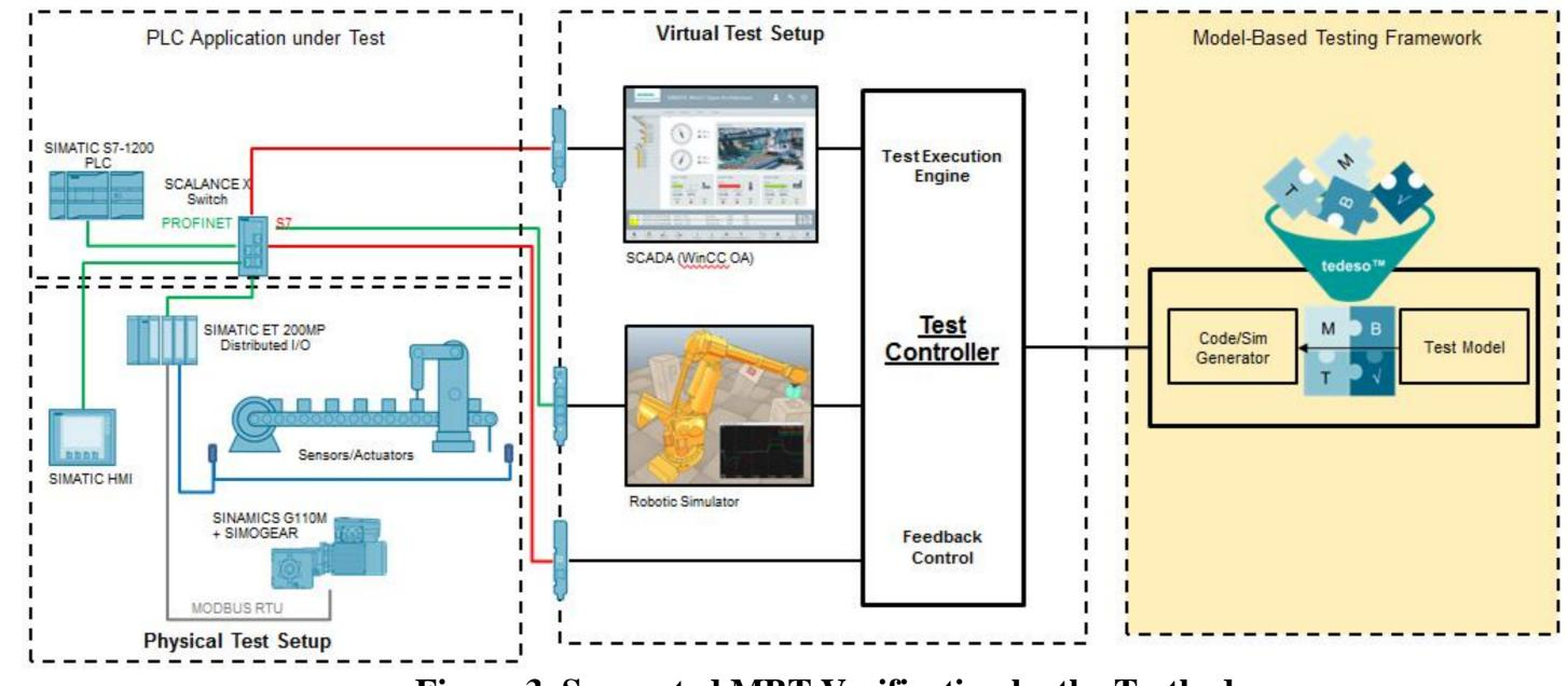
**Figure 3. Supported MBT Verification by the Testbed**
