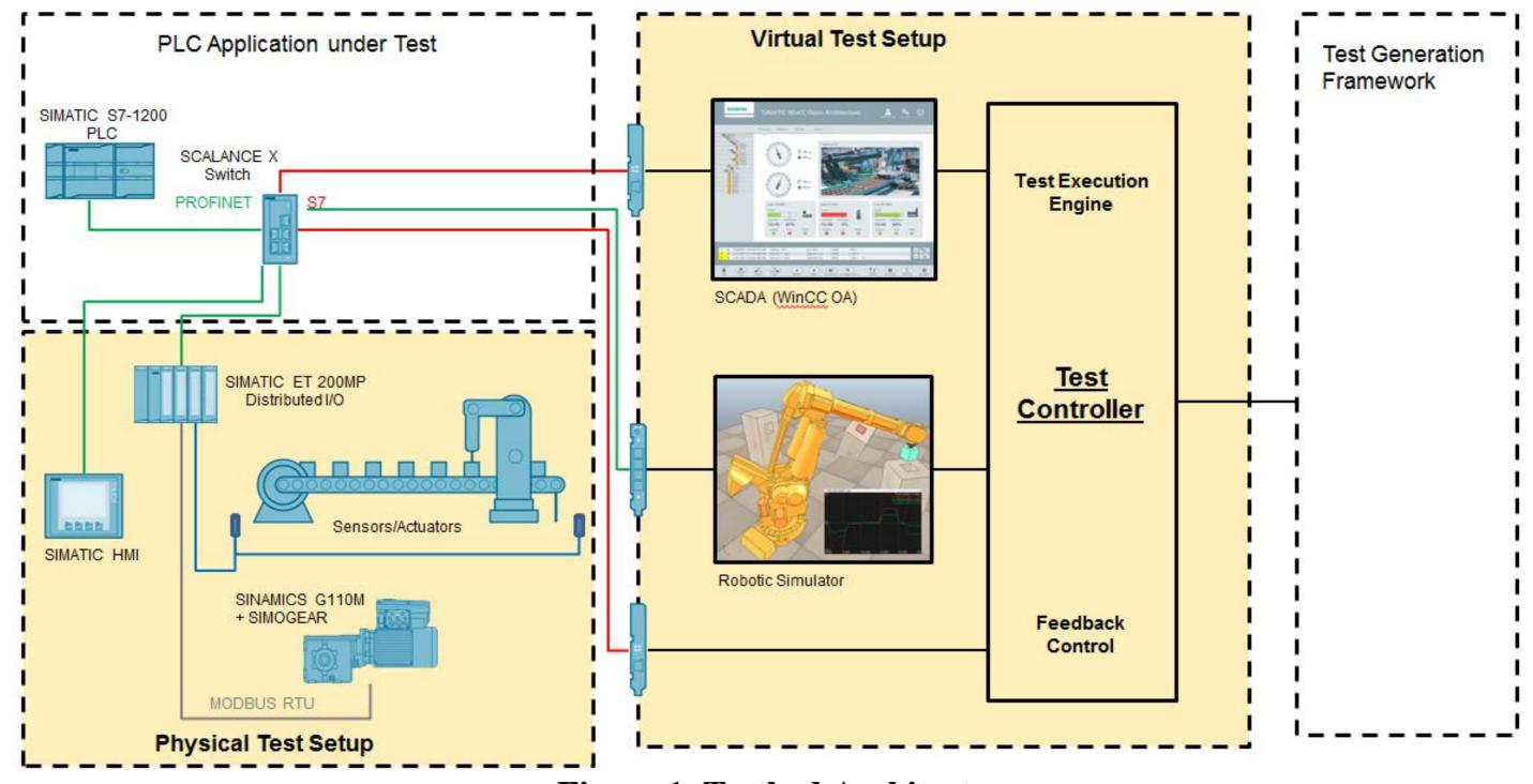
**Figure 1. Testbed Architecture**
