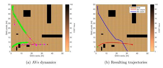
Figure 4: Simulation of the emptyWithObstacles map scenario
