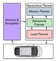
Figure 1: Control architecture of proposed benchmark.
