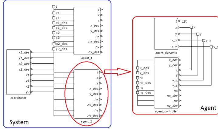
Figure 3.1: *Decentralized-style approach* for modeling autonomous systems using hybrid automata network.
