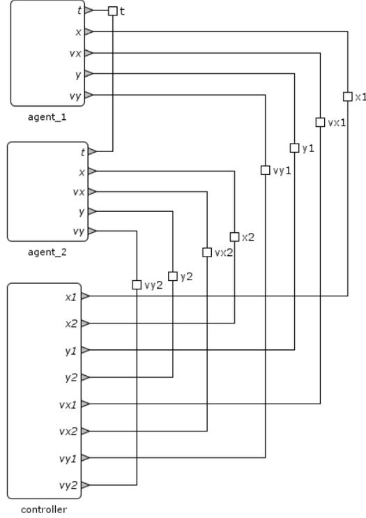
Figure 3.2: *Centralized-style approach* for modeling autonomous systems using hybrid automata network.
