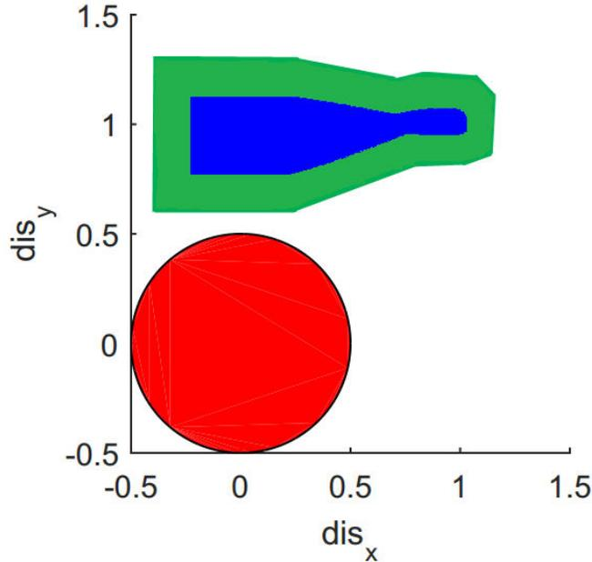
Figure 4.4: Reachable set of  $(dis_x, dis_y)$  (the green polygon),  $(dis_{xh}, dis_{yh})$  (the blue polygon) and the unsafe region (inside the red circle).
