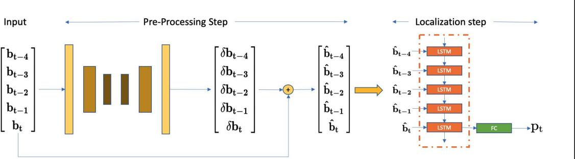
BLE RSSI characteristics vary a lot between devices. In order to make our model generalize to multiple devices without specifically collecting data and training on each one, we propose a 2 step method -
