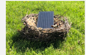
Fig. 8. An artificial hawk's nest designed by Clemson collaborators to camouflage the detection device
