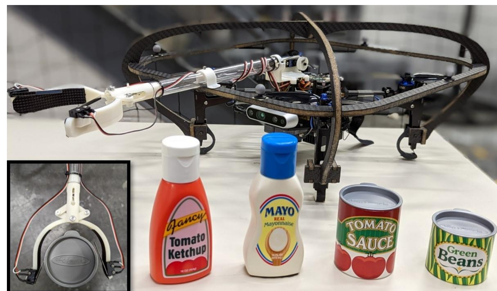
Figure 1. Compact aerial vehicle research platform with custom components. Target objects of interest are displayed in front (toy cans and bottles) and a view of the open gripper, 9.5 cm across, around a 6.5 cm diameter can.
