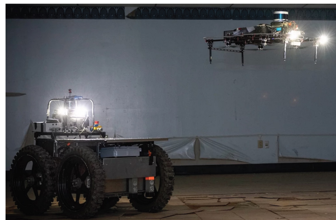
Left: Carrier robot capable of launching aerial robots (photo: CMU and OSU)
