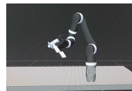
Fig. 4: Left: Simulation of the robot in OpenRAVE for planning the robot's motion.
