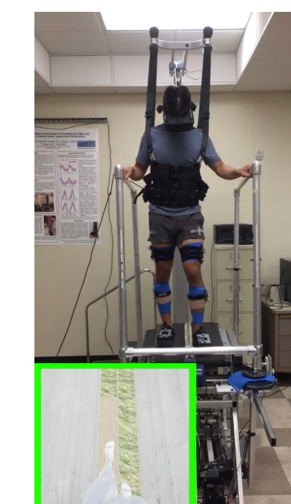
Figure 6. The VST and Oculus Rift experimental platform (left). Mean normalized activation for the GA muscle in the studied conditions: Visual and Physical (VP), Visual Only (VO) and Physical Only (PO) perturbations. (bottom)
