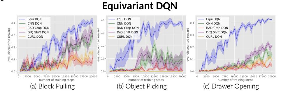
Comparison of Equivariant DQN (blue) with baselines. Results are averaged over four runs. Shading denotes standard error.
