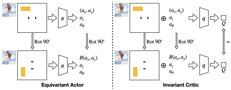
**Equivariant Actor**: When the input state image rotates, the vector in the output rotates by the rotation matrix .
