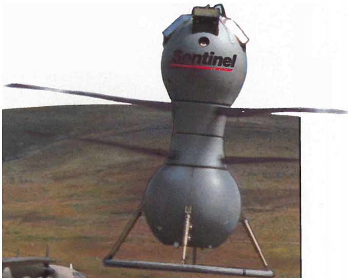
Figure 1.1: The CL-227 adopted an innovative 'peanut' design which placed its rotors at its center of gravity, its motors and exhaust at the top of the UAV, and its cameras and sensors at the bottom of the craft.
