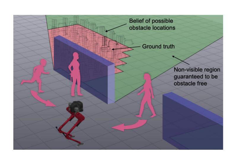
Aim 1: Risk-sensitive trajectory optimization with chance constraints for robust locomotion
