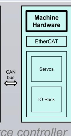
Software components in open source controller
