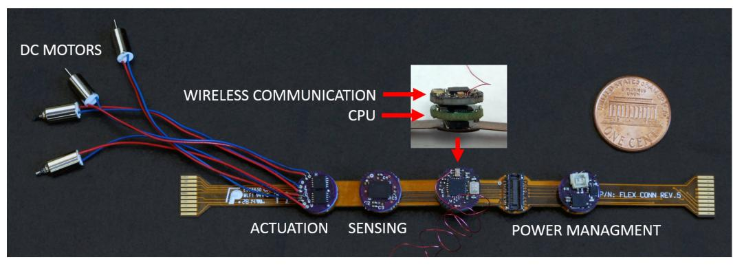
The flexible circuit with hardware modules before folding in a shape that can be integrated inside an MCR. The flexible circuit can host up to five different modules. In this case the wireless communication module is plugged on the CPU module in the central slot. The other slots are respectively hosting an actuation module, a sensing module and the power managing module.
