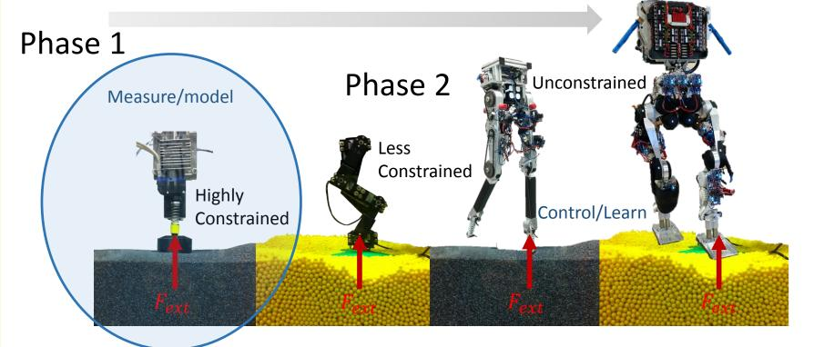
Task 1: Experimentally derive granular force laws for modeling  $F_{ext}$  through controlled experiments
