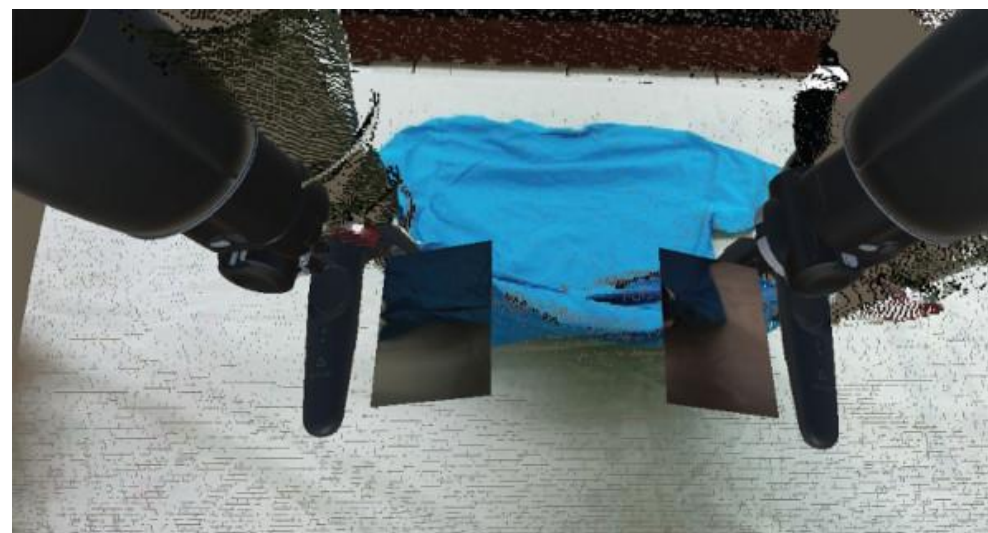
Human operator using virtual reality to fold a t-shirt using one of our preliminary interfaces.
